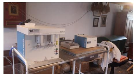
*Gluten Index is measured on a Perten Glutenomat, and express how many percent of the gluten that can be pressed through a sieve of a certain mesh size. We measure gluten index on hundreds of varieties each year.*
